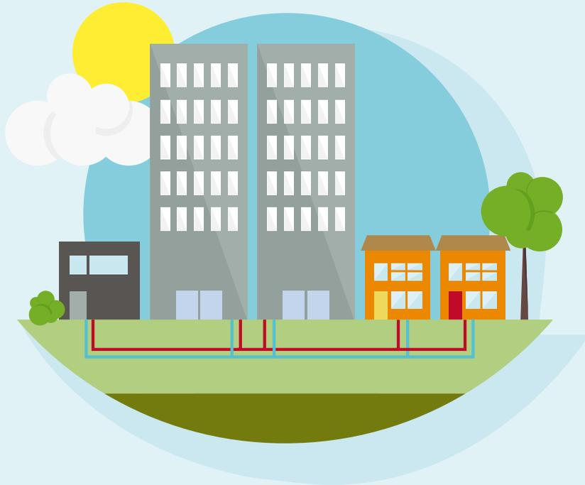
Heat networks distribute heat produced from a central point through a network of insulated pipes to both domestic and business users.
